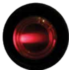
View down into the FASTspec™ vial showing fluorescence of chlorophyll.
