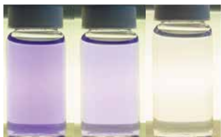
The reaction of crystal violet with sodium hydroxide slowly produces a colorless solution. This is a first order reaction.
