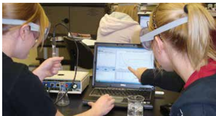
Live, high quality graphs help students visualize relationships between experimental variables. These students are observing the supercooling and freezing of a 1 mL acetic acid sample.
