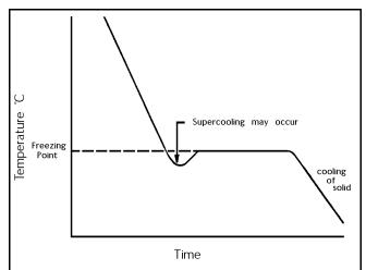
Figure 1. An idealized cooling curve. **NOTE**: The dip in the curve before it plateaus is due to **supercooling**, in which the molecules must be cooled below the normal freezing temperature before they are able to line up and crystalize.
