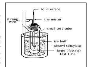
Figure 2. Set up for measuring the freezing point of Acetic acid. **NOTE**: You may be using a temperature probe other than a thermistor, and you will be using glacial Acetic acid rather than phenyl salicylate.
