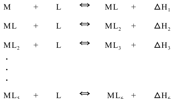
Figure 2. Diagram showing the replacement of water molecules by ammonia molecules in the nickel complex.
