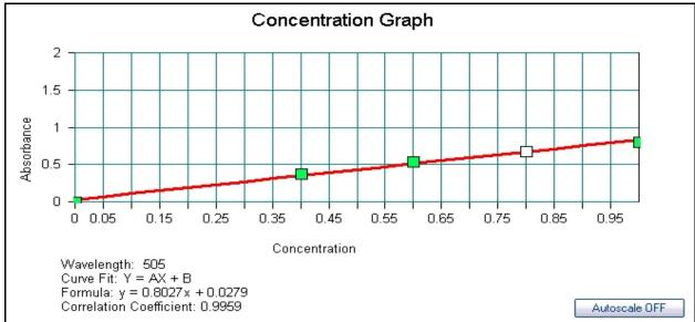
Figure 2. Sample Absorbance versus concentration graph for an  $Fe(SCN)^{2+}$  solution at 470 nm wavelength. Using the coefficient of the X term in the formula, k, we can calculate the molar absorptivity for that wavelength.
