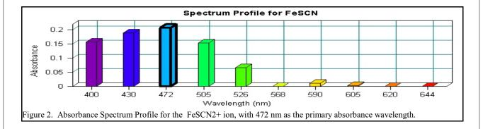
The *MicroLAB* Colorimeter Spectral Profile for the FeSCN at dilute solutions is illustrated in Figure 2, with the maximum absorbance at the 472 nm wavelength.
