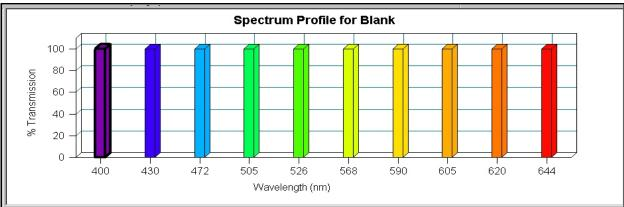
Figure 1. MicroLAB Spectrum Profile for blank illustrating the color bars for each wavelength at 100 % transmission.
