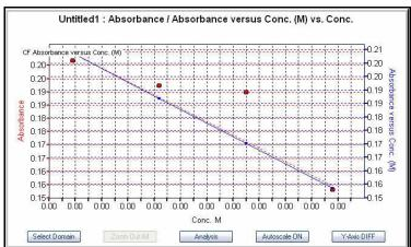
Figure 3. Graph of Absorbance of FeSCN2+ versus concentration, showing the use of the *MicroLAB* colorimeter to determine the concentration of the complex ion. This data was taken by Labworks several years ago, so does not have the resolution that the *MicroLAB* has.
