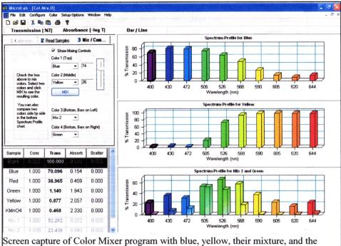
Screen capture of Color Mixer program with blue, yellow, their mixture, and the green scanned color overlayed to the right of the mixture. The mixture has been adjusted to 74% blue/26% yellow to try to match the spectrum profiles. Because they cannot be made to match, the green color is not a mixture of the blue and yellow dyes.
