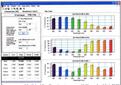
Screen capture of the Color Mixer Experiment program with blue, red and their 50/50 mixture color spectrum profiles.
