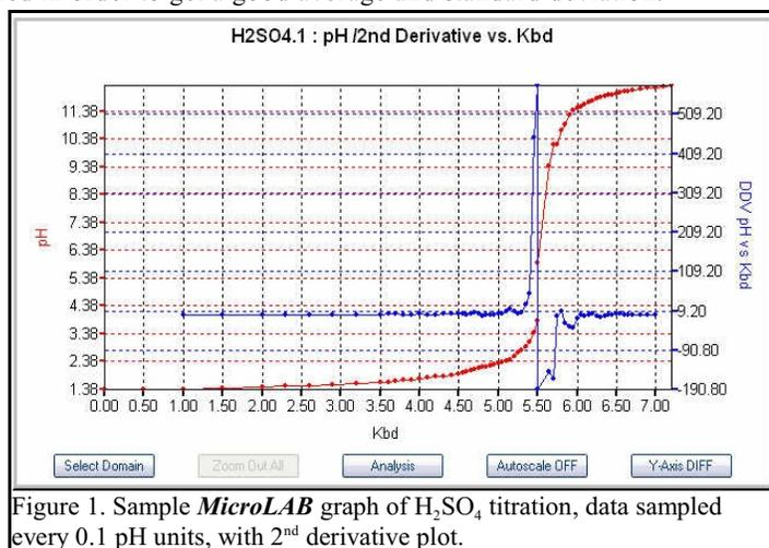
Figure 1. Sample *MicroLAB* graph of  $H_2SO_4$  titration, data sampled every 0.1 pH units, with 2<sup>nd</sup> derivative plot.
