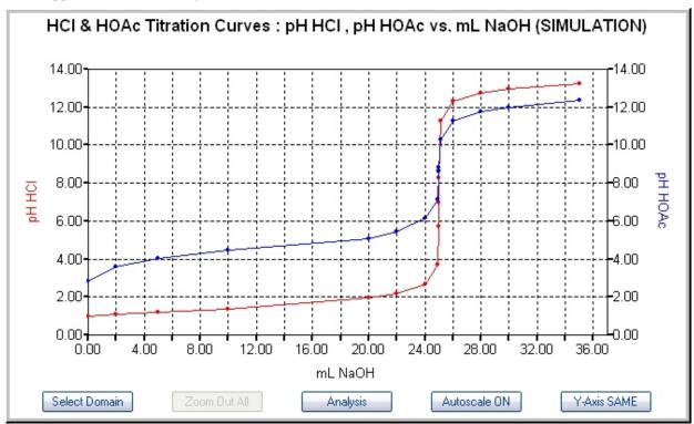
Calculated titration curves for HCl and HOAc acids with NaOH.
