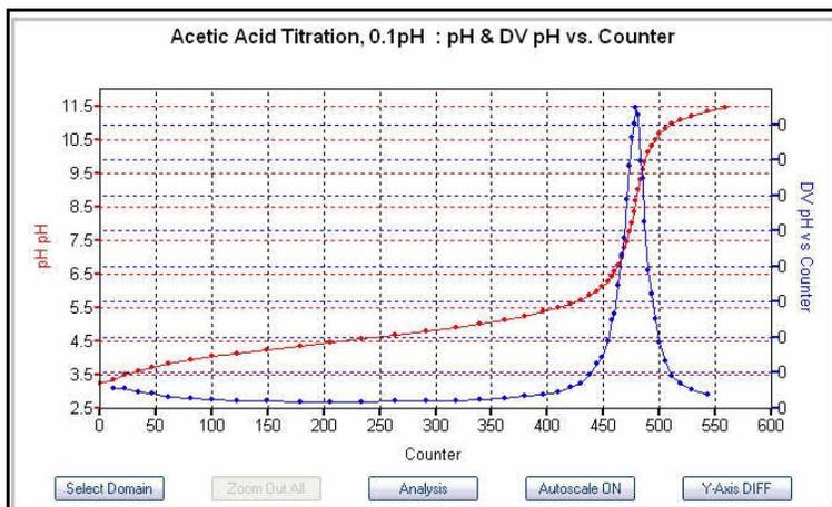
Figure 2. Classic weak acid titration curve with 1<sup>st</sup> derivative. The KHP titration curve is analogous to this.
