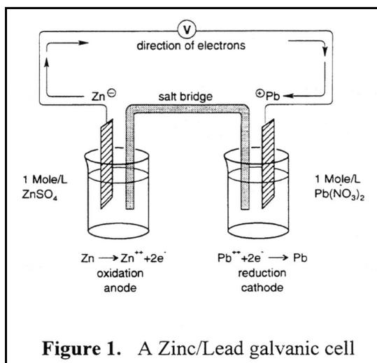
Figure 1. A Zinc/Lead galvanic cell
