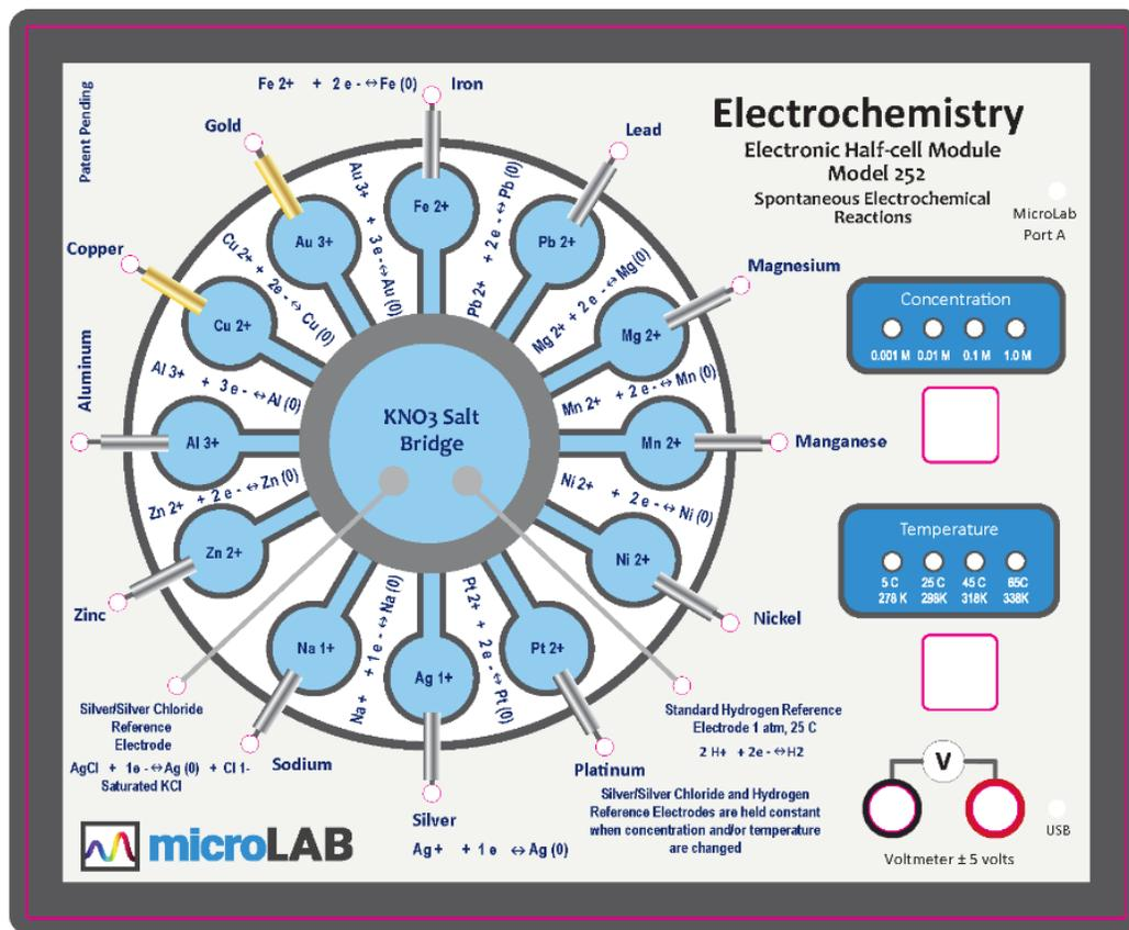
Electrochemical Half-cell module. Just transfer the black 252 voltmeter lead from outer metal case of the pH electrode BNC connector to the silver/silver chloride reference electrode pin on the Electronic Electrochemical Half-cell module.
