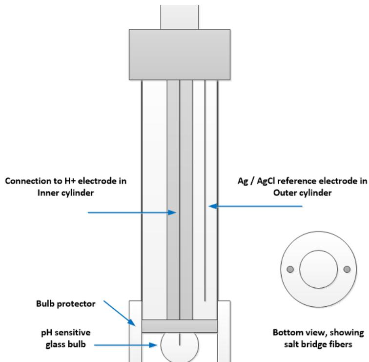
The pH electrode will fit into one of the outer wells in the Multi-EChem Half-cell module. Put about 2 mL of  $\text{KNO}_3$  salt bridge solution into the well, then insert the pH electrode.
