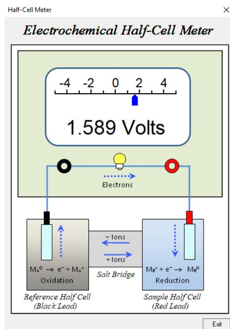
1. The electrical force exerted on electrons that travel from the negative pole to the positive pole of the battery is 1.589 volts in this example. It is presented both digitally and on an analog meter scale. The analog meter scale accents the direction of electron flow in the circuit.
