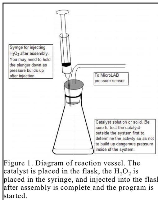
Figure 1. Diagram of reaction vessel. The catalyst is placed in the flask, the  $H_2O_2$  is placed in the syringe, and injected into the flask after assembly is complete and the program is started.
