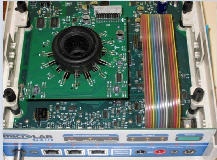
Figure 1: MicroLab's FS-522 is designed to industrial standards and assembled in a U.S. ISO-9002 certified factory. The sample cell for MicroLab's patented FASTspec™ scanning spectrophotometer shows in the foreground.
