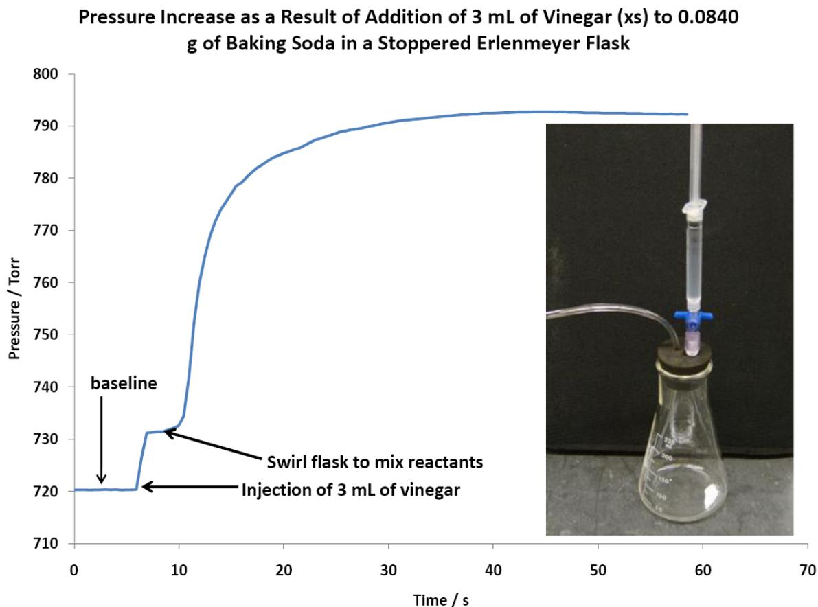
**Figure:** The plot shows a 7 sec baseline after which the vinegar was injected, but not allowed to come in contact with the sodium bicarbonate. The pressure rise between 7-8 sec is due to the vapor pressure change and the ~1% decrease in air volume from adding the solution. At the 10 sec mark, the flask was swirled to initiate the reaction. The reaction was complete one minute later.
