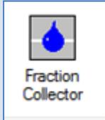
The MicroLab **Fraction Collector** program operates with the Model 226 drop counter to count drops from a chromatography column. The operator may select a number of drops for each fraction. An alarm will ring two drops before the selected number is counted, and a second alarm will ring as the selected number is counted. The operator may then change the collection vial. The counting program starts over automatically.
