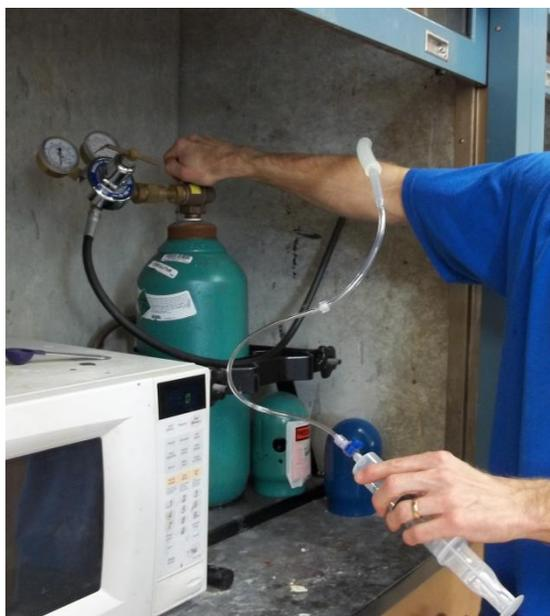
**Figure 2:** Attach pressure syringe to SF<sub>6</sub> tank.
