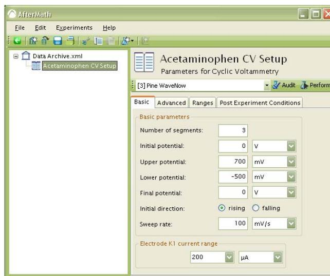
Figure 6: Configuring the Cyclic Voltammetry Parameters
