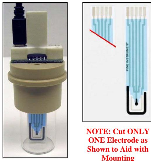
Figure 3: Student Voltammetry Cell with Disposable Screen-Printed Carbon Electrodes
