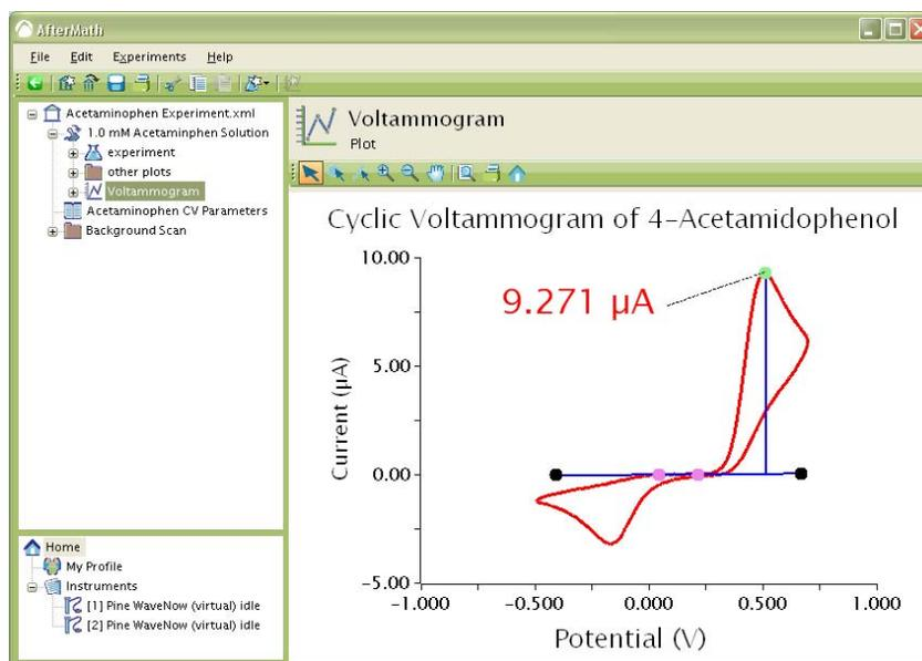
Figure 7: Example Cyclic Voltammogram of 4-Acetamidophenol in Buffer Solution
