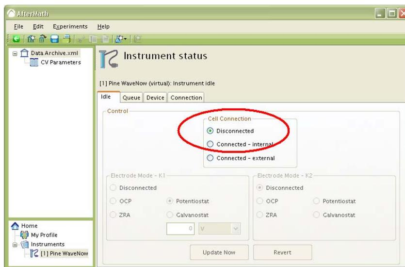
Figure 5: Setting the Potentiostat Idle Condition to Disconnected
