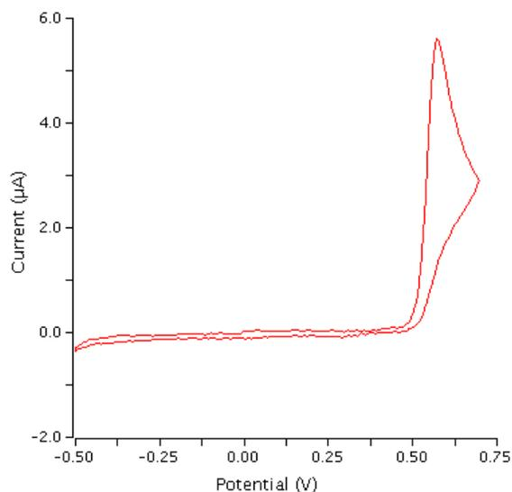
Figure 9: Voltammogram Acquired in 0.5M  $\text{H}_2\text{SO}_4$
