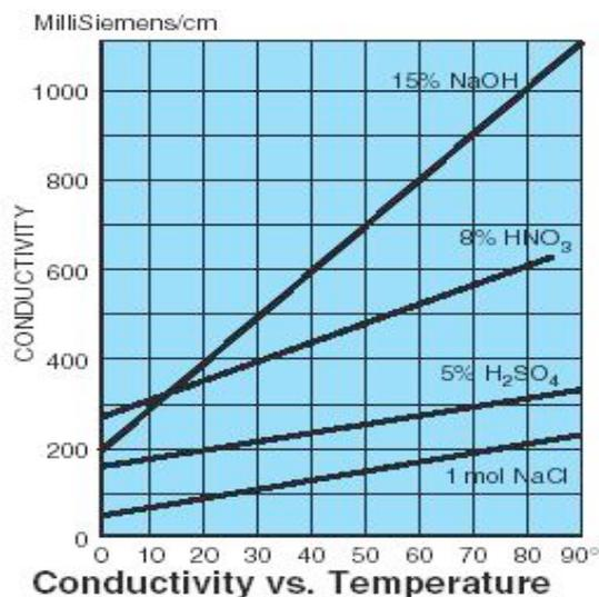
Figure 2: The conductance of a sodium chloride solution has a low sensitivity to changes in solution temperature. It makes a good conductivity standard.
