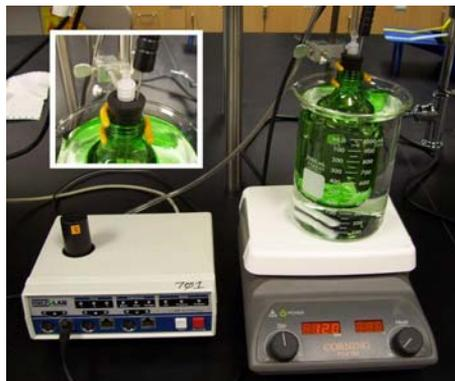
Figure 1. Setup of the ginger ale bottle showing detail of thermistor and pressure connector.
