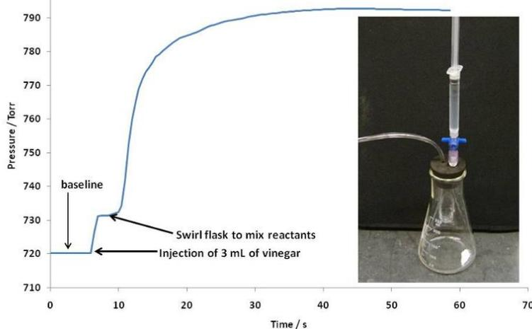
Figure: The plot shows a 7 sec baseline after which the vinegar was injected but not allowed to come in contact with the sodium bicarbonate. The pressure rise between 7-8 sec is due to the vapor pressure change and the ~1% decrease in air volume from adding the solution. At the 10 sec mark, the flask was swirled to initiate the reaction. The entire run took about 1 minute.
