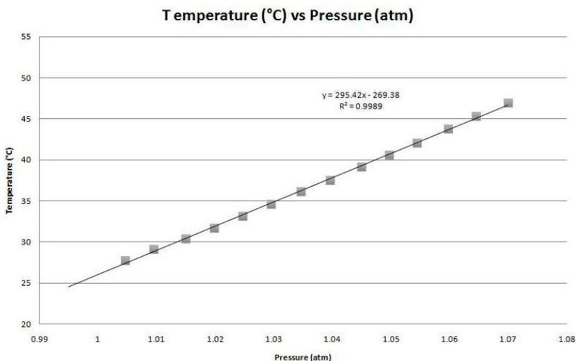
Figure 2. The improved accuracy and precision of the results obtained from measuring the temperature and pressure within the container are evident. Also evident is the sensitivity and low noise of the pressure sensor, with a range of 0.07 atm (<60 torr).
