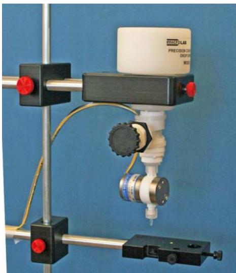
Figure 5. The Model 254 is the automated version of the constant volume drop dispenser for controlling the addition of reagent via the MicroLab software. The drop rate is set with the thumbscrew, but the dispensing is solenoid controlled via keyboard, program loop, or another sensor. The drops are counted by the Model 226 drop counter below.
