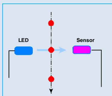
Their first design used a light beam that was broken by a falling drop, similar to the Bailey patent, although the Bailey system also measured the size of the drop. In this design, it was very critical that the light beam strike the drop exactly the same way every time. The system would not count reliably if any part of the apparatus were bumped. In this system, drop detection was indicated by a decrease in light received at the sensor.
