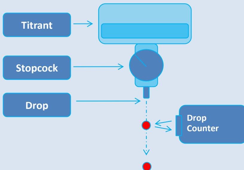
A drop counting system has three parts: A titrant reservoir, a drop generator, and a drop counter. The size of the drop is determined by the geometry of the drop-forming tip, the pressure head of the liquid above the tip, and the viscosity of the liquid. The MicroLab drop dispenser uses a wide, flat titrant reservoir to minimize the change of pressure head during a titration.
