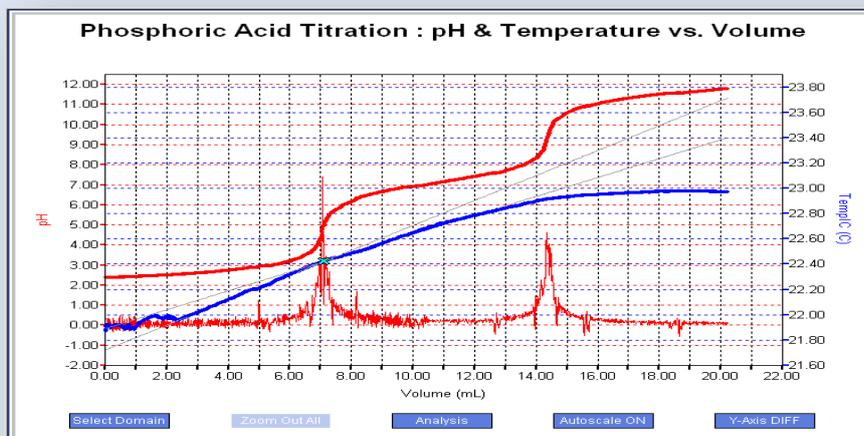
This phosphoric acid titration with NaOH took about 12 minutes and produced "text-book" data. Note the change in the slope of the temperature curve after the first end point. The heat of reaction for neutralization of the first hydrogen is larger than that for the second hydrogen.
