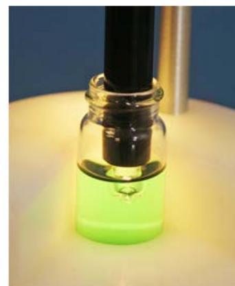
10-watt variable power heater & sample illumination module
